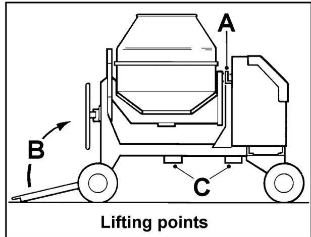
Spread the fork tines and carefully position them so that they pass through the brackets **(C)** that are attached to the mainframe.
